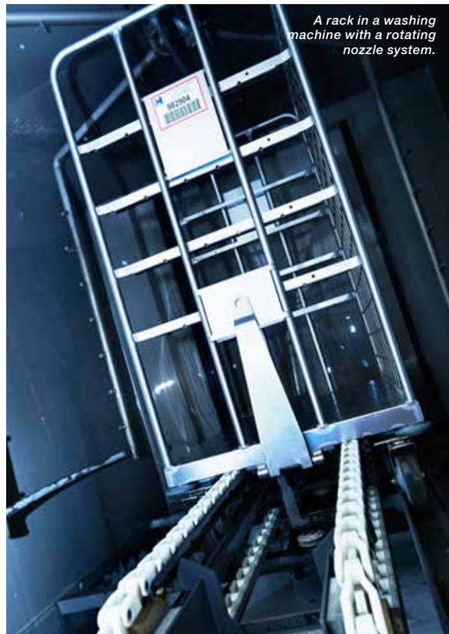
SEMI-STAAAL's crate/ lid washer seen from the inside.
