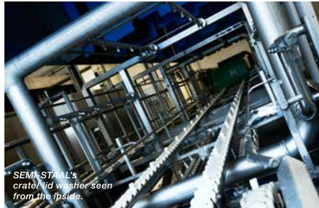
A rack in a washing machine with a rotating nozzle system.
