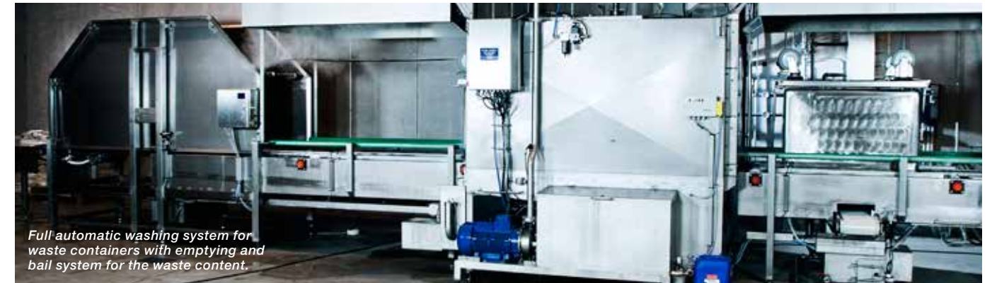
After the waste content is emptied into a bailer, the containers are automatically checked if they are empty before they are forwarded to the washing system.
