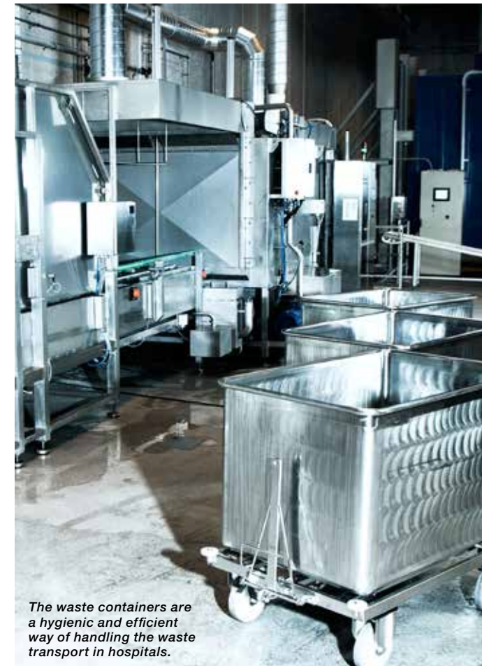
Full automatic washing system for waste containers with emptying and bail system for the waste content.
